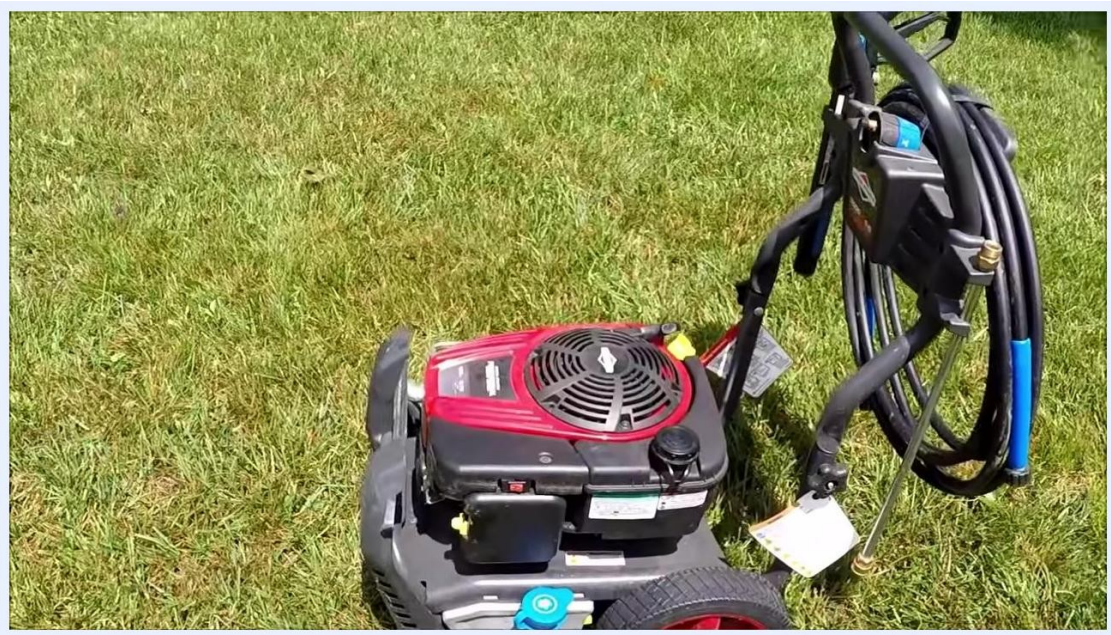
Top view of the engine and starter cord with the oil cap reinstalled, the pressure washer resting on grass.
