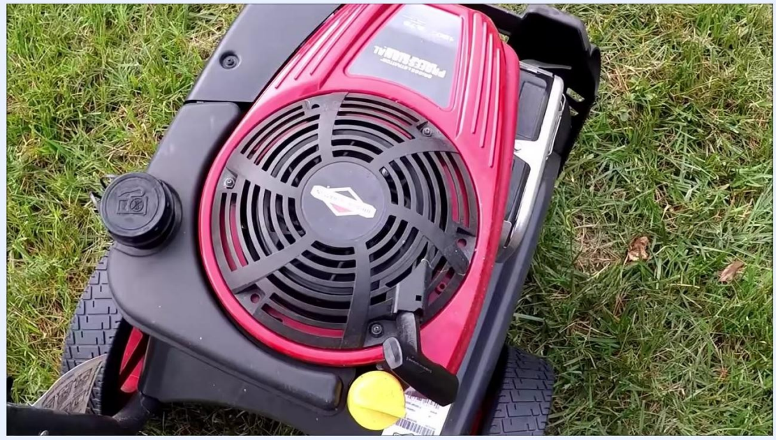
Engine top with the yellow oil fill cap, black fuel cap, red cover, and pull start handle on grassy ground.
