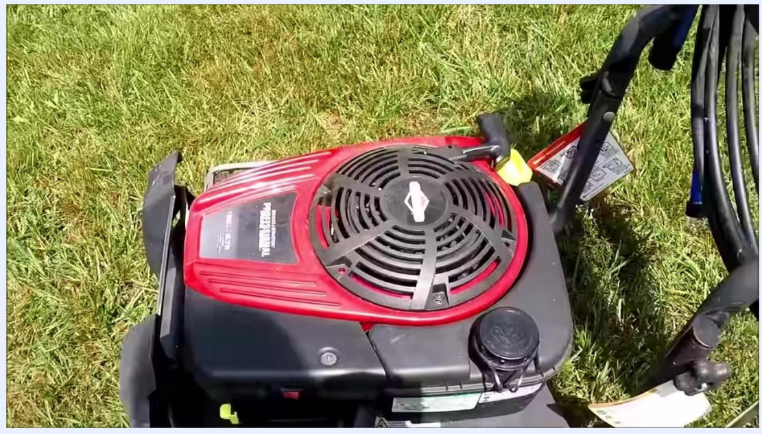
Top view of the pressure washer engine showing the red engine cover, pull handle, and fuel cap, with the starter cord in use on grass.
