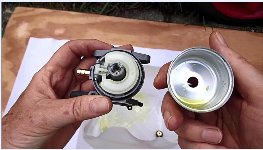
Close-up of the carburetor and float bowl, both appearing clean, with the float mechanism and brass jet visible.
