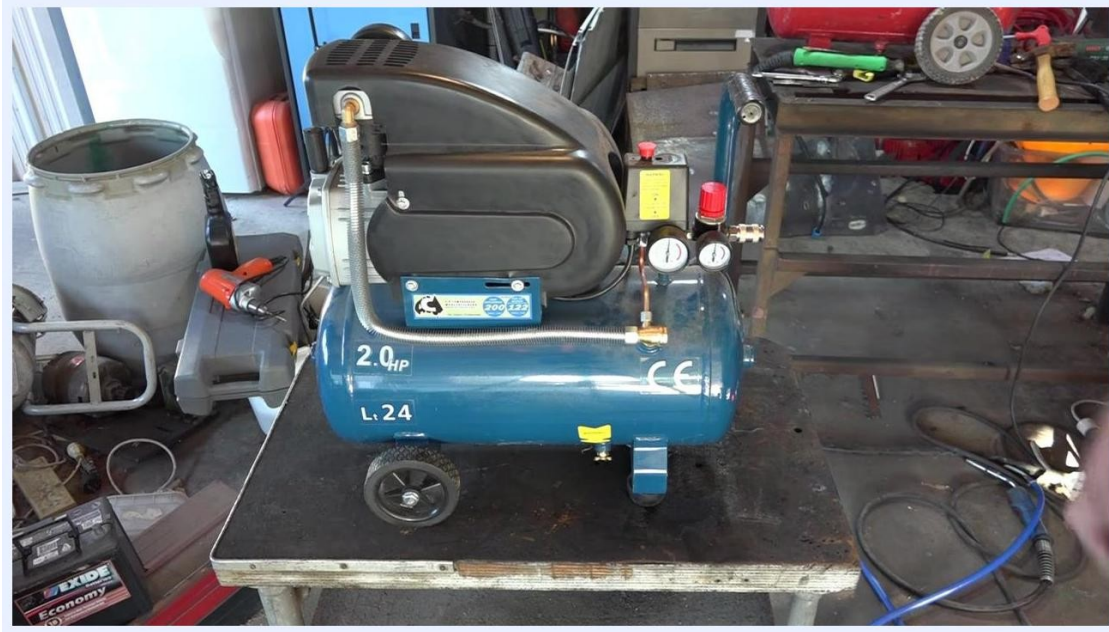
Pressure switch housing with warning label, red ON/OFF button, red regulator knob, and dual pressure gauges
