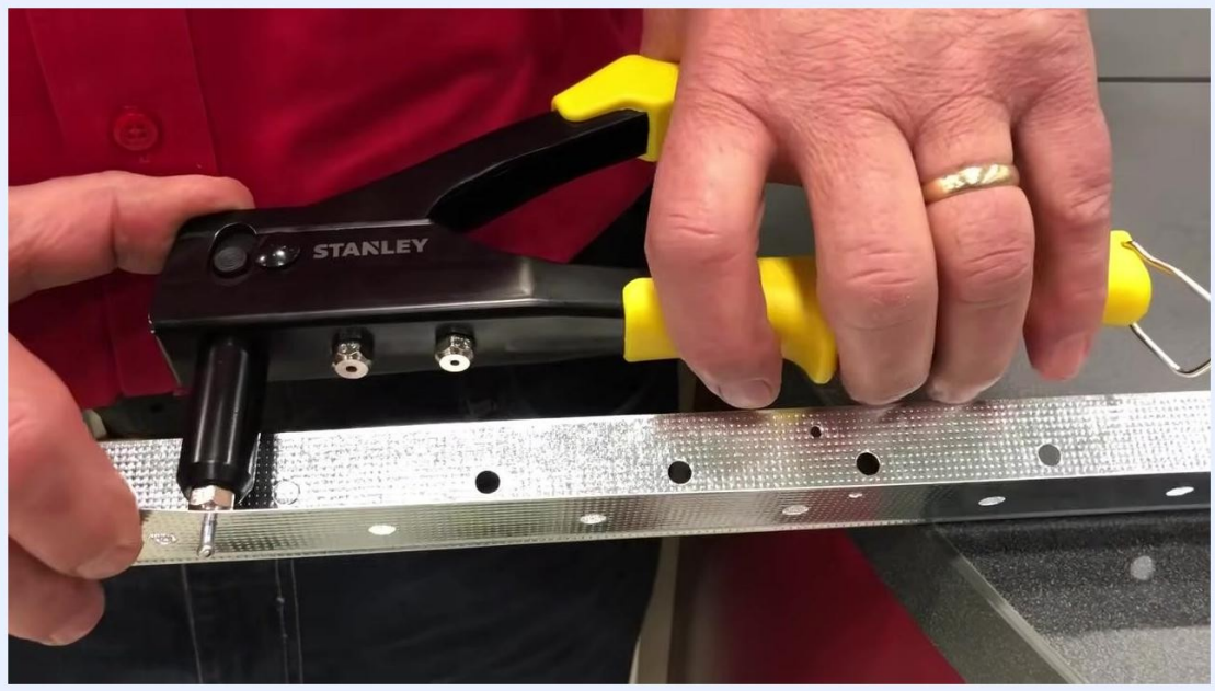
Yellow-handled rivet gun and a rivet being prepared for insertion above the metal strip
