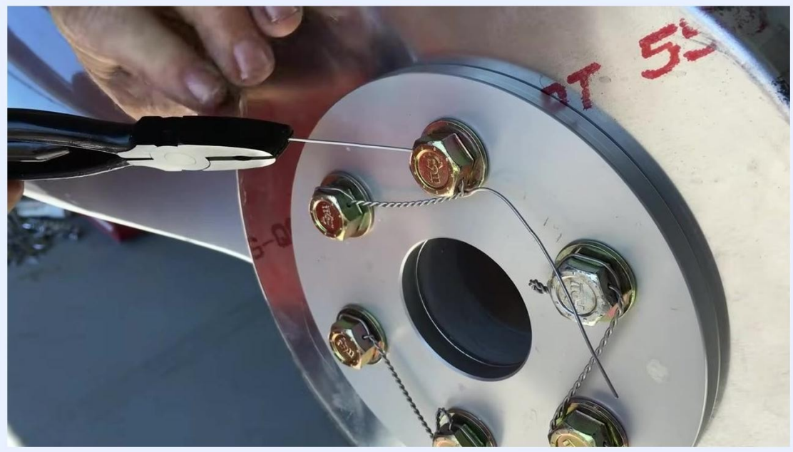
Inspecting the tightness of the safety wire after pulling it with pliers
