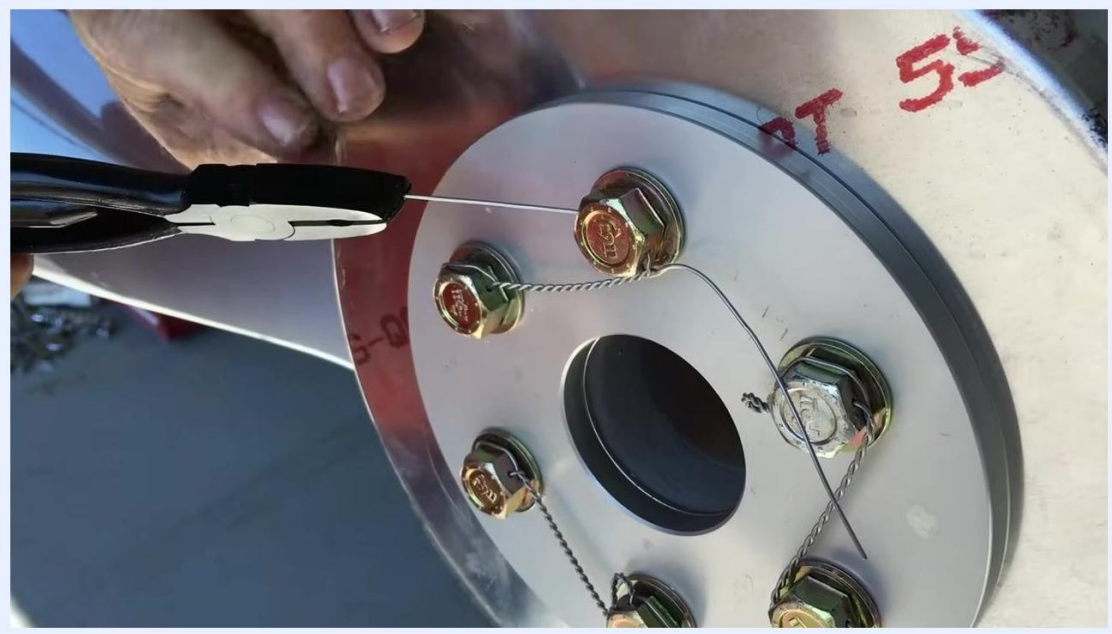
Using safety wire pliers to pull the wire tight after threading it through the bolt head
