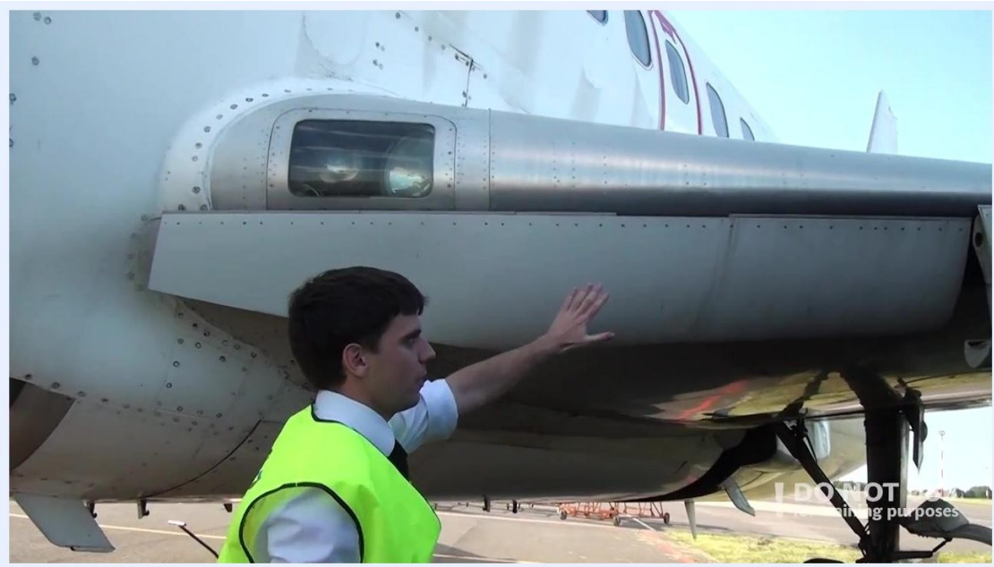
Inspector reaching up to inspect the wing root, leading edge flaps, and exterior lights.
