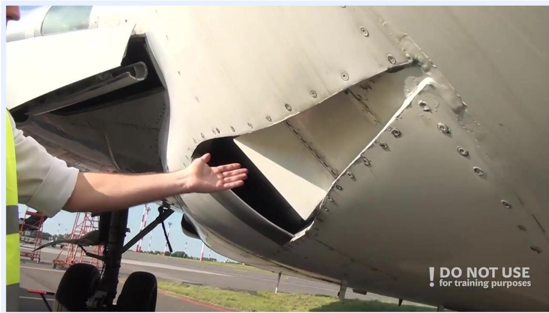
Person standing near the engine nacelle, reaching up to inspect the leading edge flaps of the wing.
