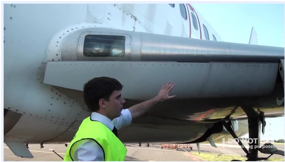
Person standing next to the right front fuselage, inspecting the pressure relief disc and surrounding markings.
