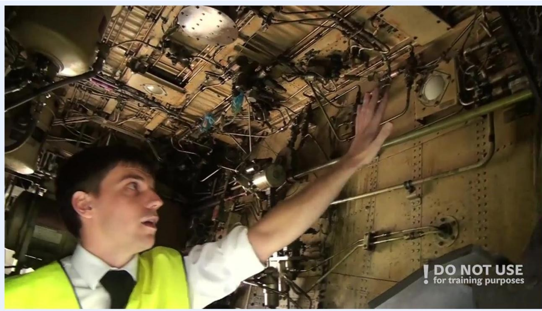
Inspector reaching up to inspect the trailing edge of the wing and flaps.
