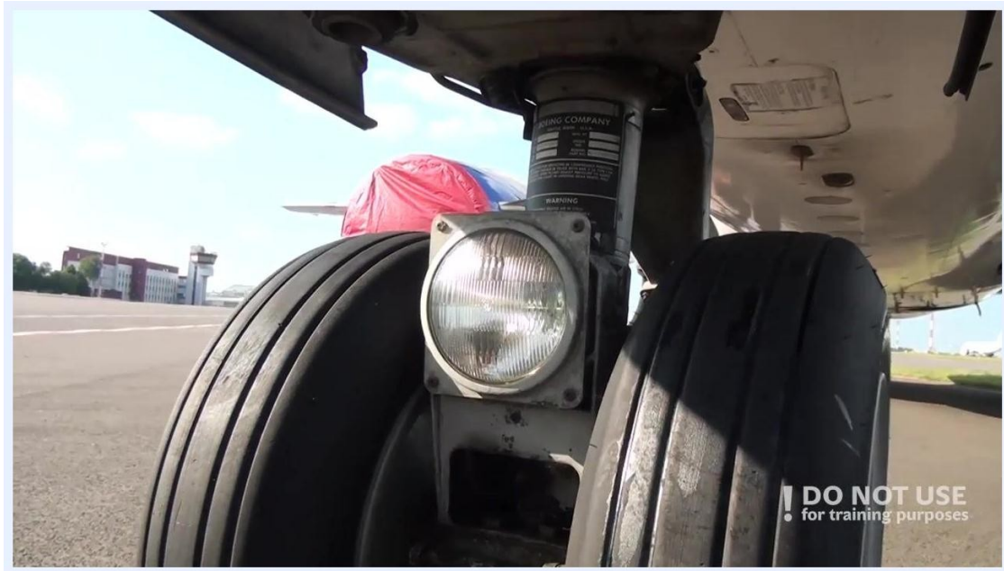
Close-up of the nose gear assembly, showing the wheels, exterior light, and steering mechanism.
